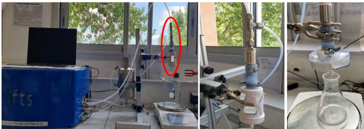
Fig. 2. Adaptation and adjustments of water purification lab cartridges into IFTS LLDP porometer
